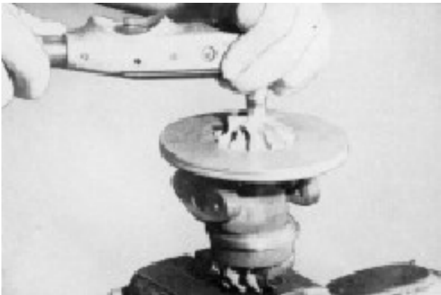
B. Remove the compressor rotor. Press the shaft out if the rotor is stuck.
